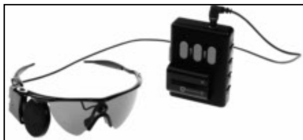
The "bionic eye" works thanks to a pair of glasses with an attached miniature video camera and a processor on the wearer's belt
